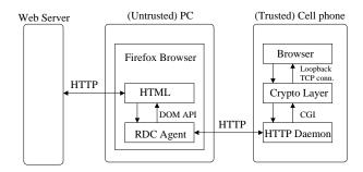
Figure 3: Architecture diagram showing components running on both the untrusted PC and the trusted personal device
