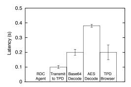
Figure 6: Latencies of the individual components of our implementation (averaged over 20 trials). Error bars show standard deviations. TPD abbreviates Trusted Personal Device—in this case, the Motorola E680 smart phone.
