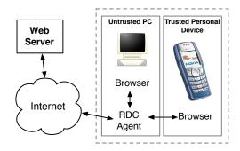
Figure 1: High-level overview of our system for split-trust browsing
